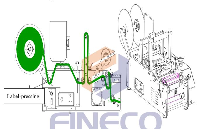
1.step1 :winding the label according to the diagram above, loose the traction device when the label goes through and Fasten it after that.
